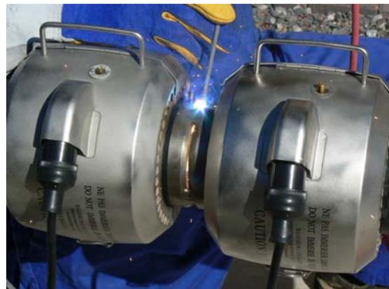
**Clean Operation:** Operated by clean electrical energy *Hot Coils®* eliminate the dangers of open flame, explosive gasses and high heat hazards associated with propane. The operator is not exposed to the exhaust gasses or the burning of any pipe coatings or oil film.
